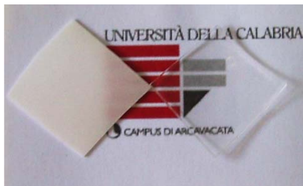
Fig. 1 Photo of the dense PDMS/ \beta CD (on the left) and PDMS (on the right) membranes
